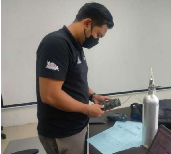
Figure 11.14 Site Calibration Portable Gas Detector at NIOSH Regional Office NIOSH
