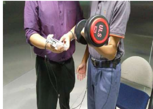
Figure 9.26 Muscle activity measurement and fatigue assessment using electromyogram (EMG) device
