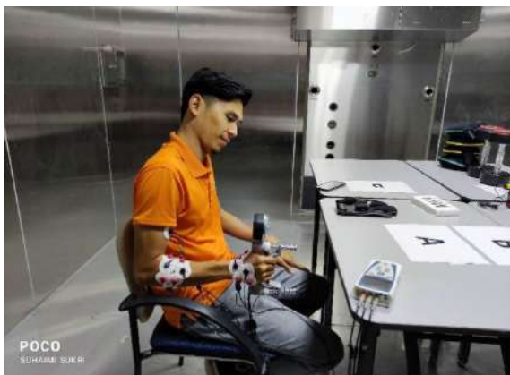
Figure 9.33 The measurement of muscle activity and muscle activation profile during gripping exercise
