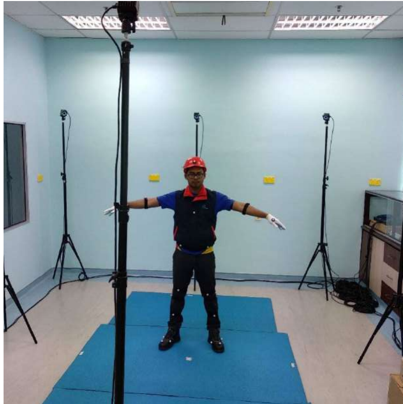
Figure 9.8 Optical motion capture systems have become increasingly widespread in human factors & ergonomics, biomechanics and sports science studies.
