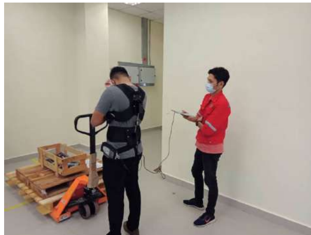
Figure 9.47 The lumbar spine motion monitoring was utilised to measure the effectiveness level of ergonomics control practised within industries
