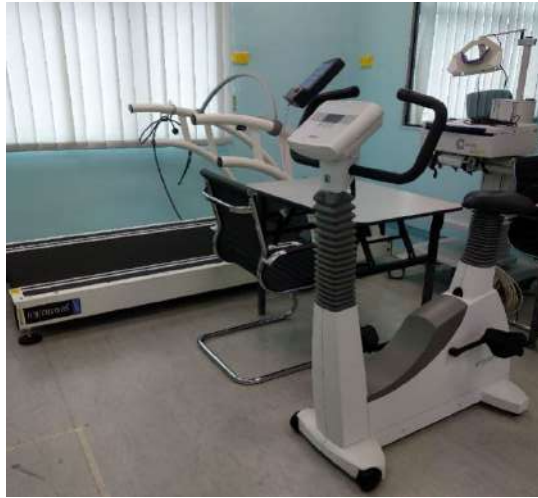
Figure 9.13 A medical treadmill and ergometer simulate the physical activities for cardiopulmonary and performance metabolic tests
