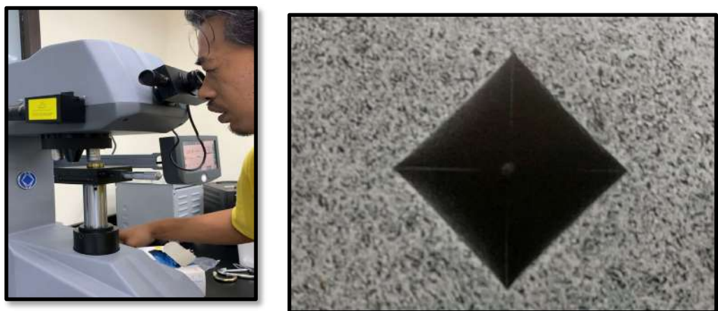
Figure 13.7 Hardness Testing & Vickers Hardness Test Analysis
