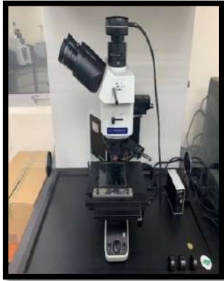
Metallurgical Microscope with Microscopy Camera & Analysis Software
