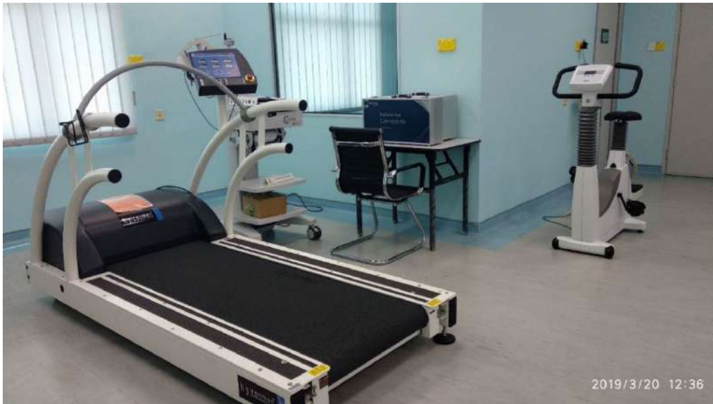
Figure 9.11 Spiroergometry and ergometer systems for evaluation of human metabolic system while under physical stress
