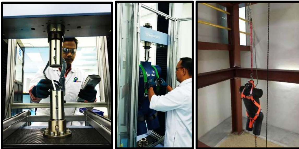
Figure 1.3 1) Static strength test for connector, 2) Static strength test for full body harness, 3) Dynamic performance test for the full body harness
