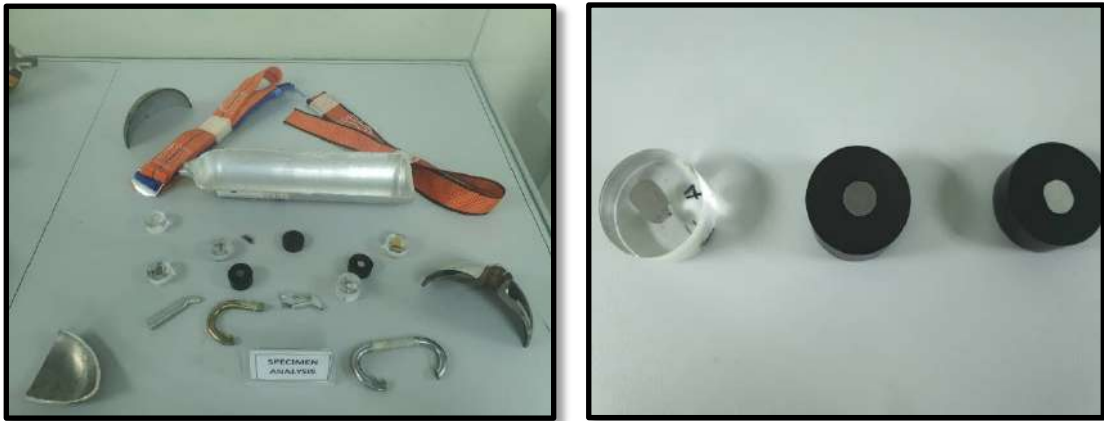
Figure 13.5 Metal parts of full body harness & Sample of metallurgical analysis
