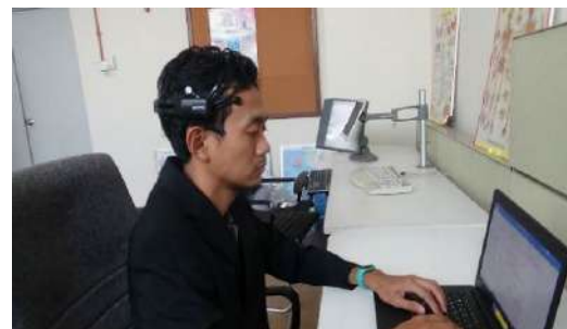
Figure 9.16 The measurement of brain activity using a portable electroencephalogram (EEG)
