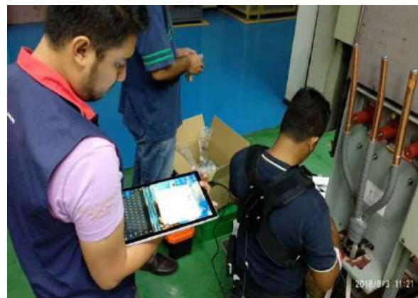
Figure 9.34 Measurement of low back disorder risk among cable jointer
