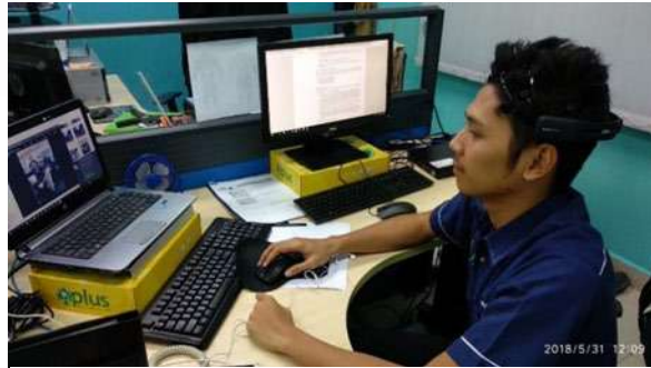
Figure 9.18 The measurement of brain activity using a portable electroencephalogram (EEG) for sedentary worker
