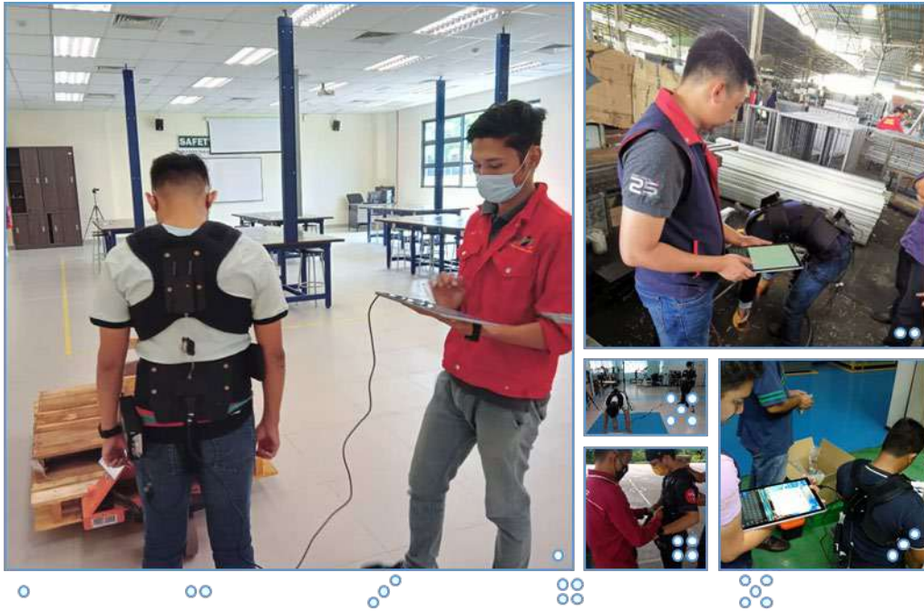
Figure 9.4 The application of the lumbar motion monitoring test in the industrial setting
