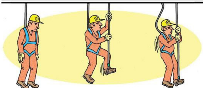
Figure 3: Climbing the On-site Equipment to Release the Pressure
